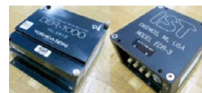
Data logger to check the status of equipment being transported
